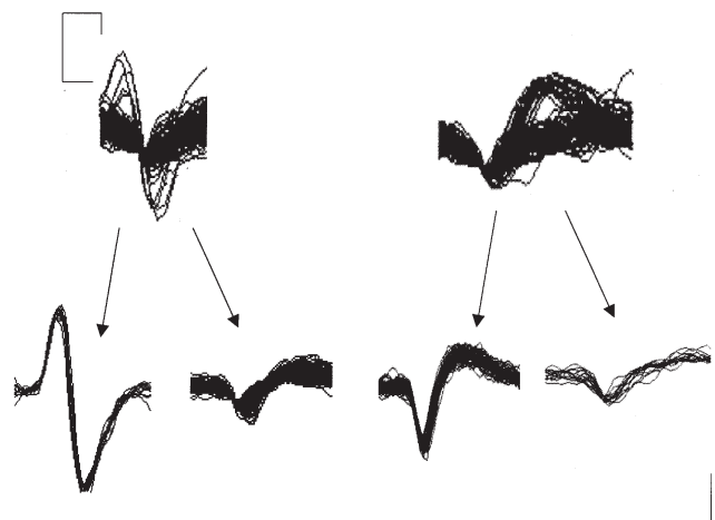
Fig. 1. Digitally derived waveforms showing the firing of four simultaneously recorded VTA neurons from two individual microwire electrodes from a 4 \times 2 array. Waveform calibration: 80 \mu V, 0.5 ms.
